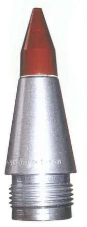
The V-5K fuze is intended for use on the S-5K, S-5KO, S-5MO and UAR-57TB unguided aicraft rockets. It serves to ensure their safety during handling and firing and to detonate the rocket's warhead on impact with a target. The fuze is nose, impact with instantaneous and inertial action, non-boresafe type.
