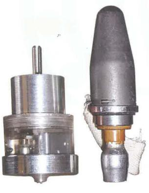
The fuze is a piezoelectric, nose-base type with percussion-instantaneous action, distant arming and a self-destruction mechanism.
