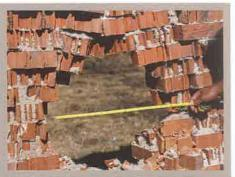
Penetration: Width 540 mm Height 780 mm
