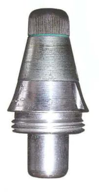
The O-4M fuze is intended for use on 82 mm fragmentation mortar bombs fired from the BM82, 2B14, and for use on the OG-7 fragmentation grenade for the RPG-7V. It serves to detonate the warhead on impact with the target. The fuze is a nose impact type with two settings – for instantaneous (fragmentation) and inertial (HE) action, semi-boresafe, with distant arming.
