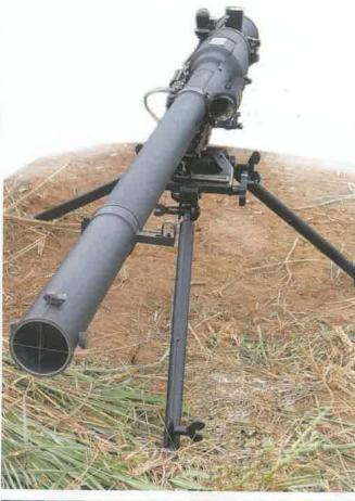
SPG-9 is primarily an anti-armour weapon firing a 73 mm high-explosive anti-tank warhead to ranges exceeding 1,300 m.
